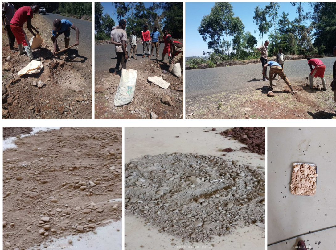
Figure 2. Photo of Sampling and preparation of samples for laboratory tests.
