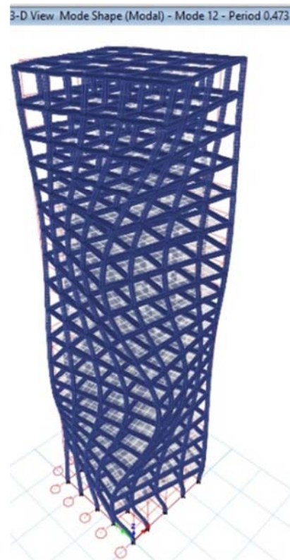
Figure 14. Mode shapes for 12th mode for twenty storey building using rectangular columns.
