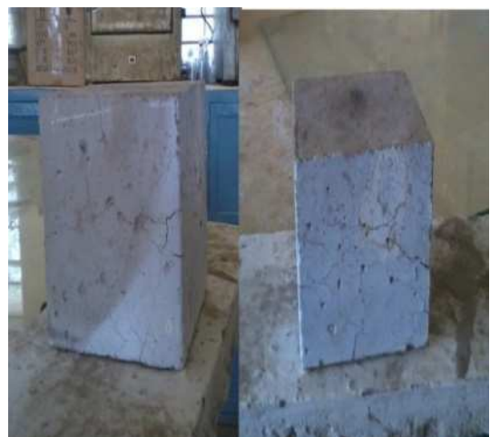
Figure 20. Concrete specimens subjected to 800°C.
