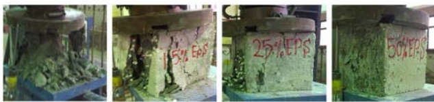
Figure 7. Failure modes under compression test.
